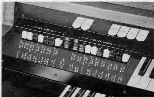
Figure 1-8. Drawbars & Control Tabs (Partial View)
